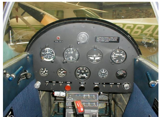
The basic factory-installed instruments, meeting VFR requirements, consist of altimeter, magnetic compass, airspeed indicator, tachometer, oil temperature and pressure gauges, and a fuel gauge.
