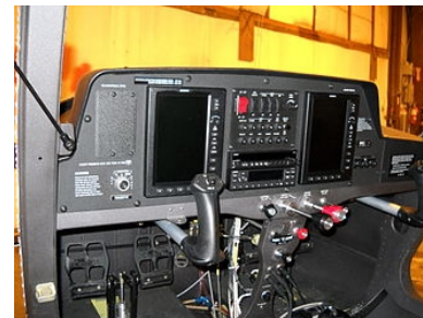
Cessna 162 Skycatcher Instrument panel. This aircraft is a factory demonstrator and has the second optional EFIS display installed.
