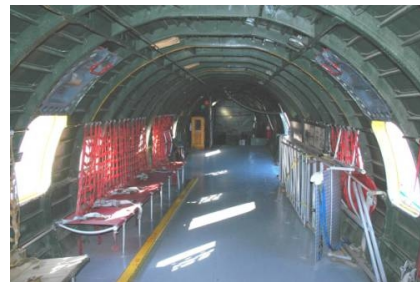
The cargo area in the C-46 was 48 feet long, 9 feet, 10 inches wide, and 6 feet, 8 inches high.
